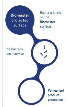
In typical tests, GPPS treated with Biomaster reduced the levels of E.coli and Staphylococcus aureus by over 99% achieving ISO 22196:2011.
