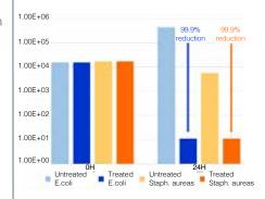
ISO 22196 results comparing bacterial load on an untreated surface with a Biomaster protected surface
