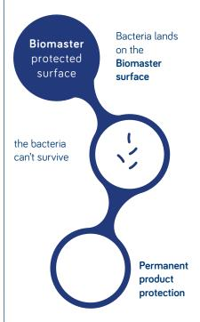
In typical tests, PC/ABS treated with Biomaster reduced the levels of E.coli and Staphylococcus aureus by over 99% achieving ISO 22196:2011.
