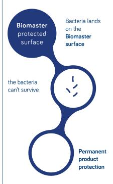
In typical tests, PVC treated with Biomaster reduced the levels of E.coli and Staphylococcus aureus by over 99% achieving ISO 22196:2011.
